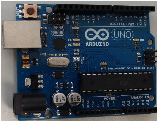
Figura 9.1: Tarjeta Arduino Uno
