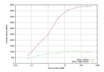
Figure 3: Transfer speed from one GPU to another using GPUDirect and via main memory
