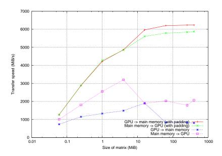
Figure 2: Transfer speed from GPU to main memory, and from main memory to GPU, with and without padding, for different matrix sizes
