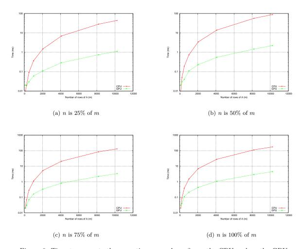
Figure 6: Time to compute the operation  $y = \alpha Ax + \beta y$  on the CPU and on the GPU
