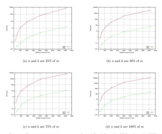
Figure 4: Time to compute the operation  $C = \alpha AB + \beta C$  on the CPU and on the GPU
